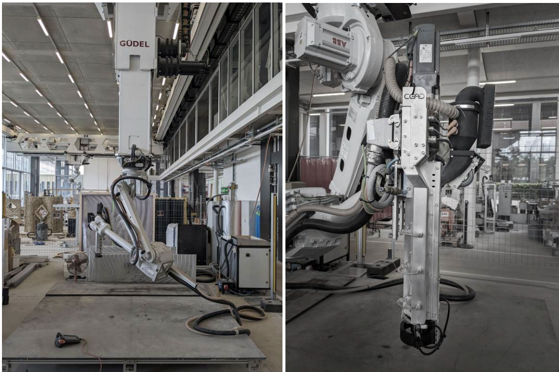
Figure 7. ABB 4600 Robotic Arm attached to a gantry (left picture) and CEAD thermoplastic extruder (right picture).
