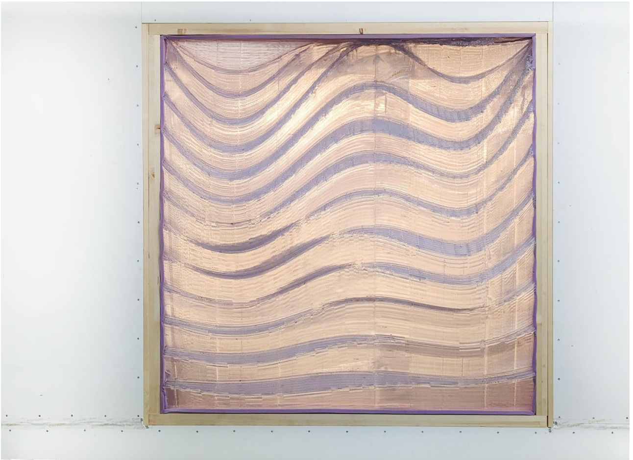
Figure 11. a) Fabrication of the fourth iteration with height of 1998 mm; b) Back view of the 3D-printed facade panel; c) Front view of the panel.
