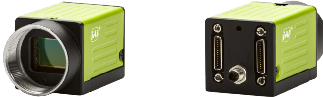
Figure 3.5: GO-5000M-PM camera by JAI; front and back view with two CL ports [7]
