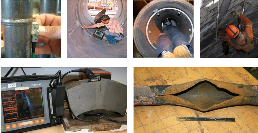
Figure 1.1: Industrial inspection. Top row: NDT of industrial structures presents many challenges: manual work, need for reliability and expert knowledge, limited accessibility and safety issues. Bottom row: Typical ultrasonic NDT system with pulser/receiver, sensor probe and display device, scanning a metal test structure with buried defect; burst tube, which demonstrates possible consequences of missed defects at inspection. (Image sources: ALSTOM Power Services, Aqualified LLC, RIGCOM Access.)
