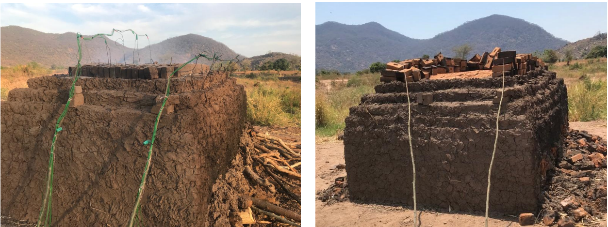
Figure 2.7: The clamp during (left) and after the firing process (right).
