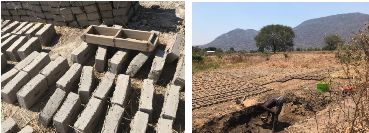
Figure 2.4: Moulding and drying of raw bricks.
