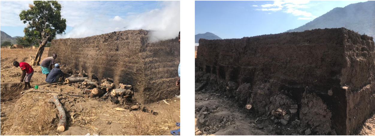
Figure 1.6: Burning of the stacked bricks using fuelwood.
