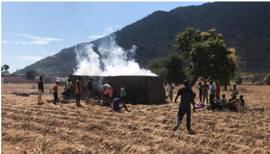
Figure 2.11: Hot flue gases accelerate the transport of heat from the burning chambers to the top surface.
