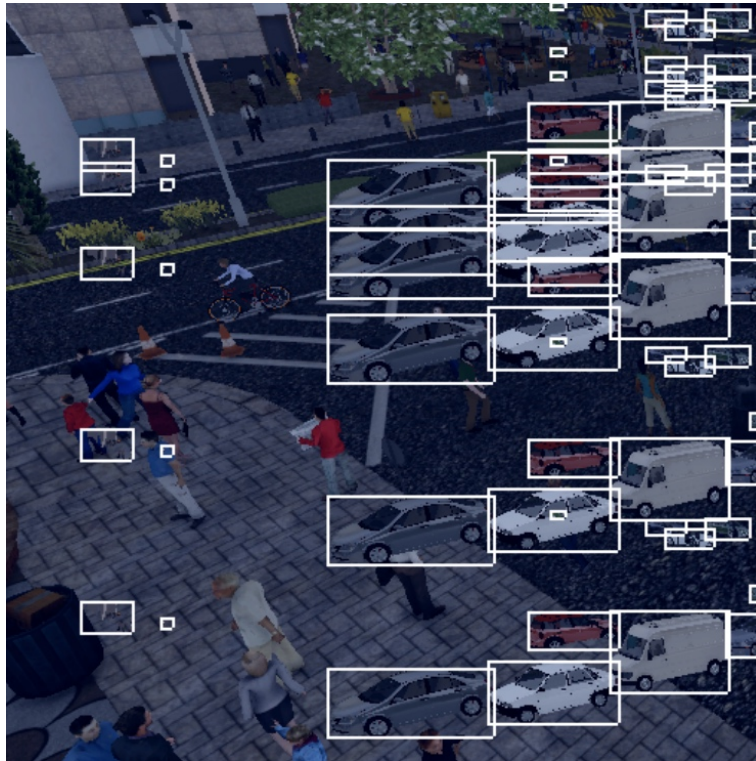
Figure A.4: Several groundtruth source cars are pasted onto the source image in order to mimic the overlaps, occlusions, and number of cars in the Cityscapes dataset
