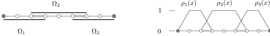
Figure 10.3: Domain decomposition on the discretised geometry. (left) Partitioning of the computational domain using \xi = 1 . (right) Definition of the (unit partitioning) weight functions \rho_k(x) which guarantee a “conservation of the solution” in the overlaps.
