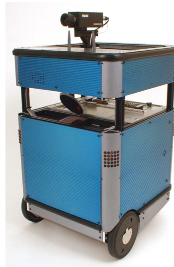
Figure 4: Pygmalion, the robot which was used in the experiments. It is a VME based system with a six axis robot controller. The processor board carries currently a PowerPC at 100MHz. Besides wheel encoders and bumpers, the sensory system includes the laser range finder and the CCD camera discussed in the second chapter.
