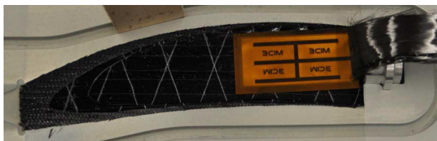
Figure 5.7: Picture of the piezoelectric patch embedded in the blade during the lamination process.
