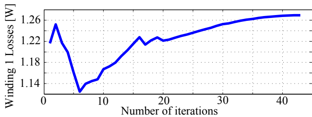
Figure 8. Foil-to-square-conductor Method Iteration, for flyback-transformer as specified in tab. I: Winding losses in the foil winding P_{foil,totk,k} (see 21) with advancing iteration.
