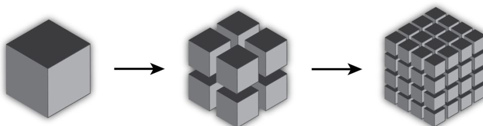
Figure 1.1: The overall surface area per material volume rises in non-linear manner when objects are sliced into smaller and smaller pieces.
