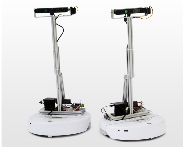
Figure 3.3: The two low-cost ( < 600\$ ) robots used in our evaluations: Each robot consists mainly of a differential drive base (iRobot Create), an RGB-D sensor (PrimeSense), an ARM-based single board computer (ODROID-U2), and a dual band USB wireless device.
