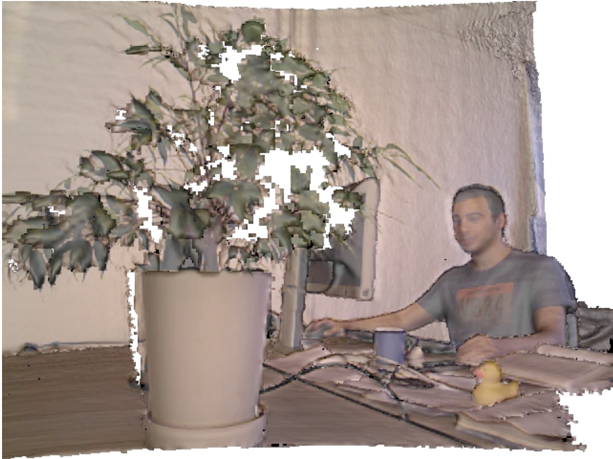
Figure 2.16: A frame of the KinectFusion output running on an Amazon GPU instance in Ireland.
