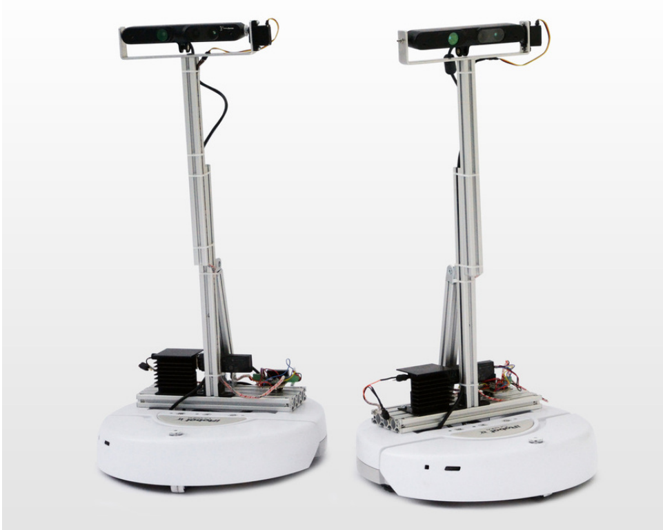
Figure 2.15: The two low-cost ( \sim 600\$ ) robots used in our demonstrators: Each robot consists mainly of a differential drive base (iRobot Create), an RGB-D sensor (PrimeSense), an ARM-based single board computer (ODROID-U2), and a dual band USB wireless device.
